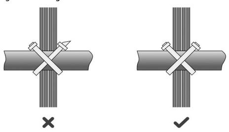
o When cables need to be bent, bind them first but do not tie cable ties within the bend. Otherwise, stress may be generated on the cables and cause the wires inside to break, as shown in Figure 7-3.
