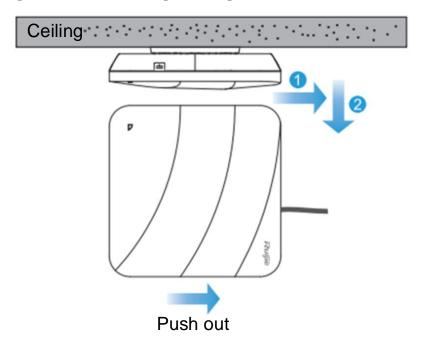
(2) If the AP is installed against a wall, hold the AP in your hands and push it upward and away from the bracket in the LAN port direction.
