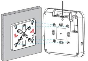
⚠ Install the Ethernet cables before mounting the AP on the bracket.
